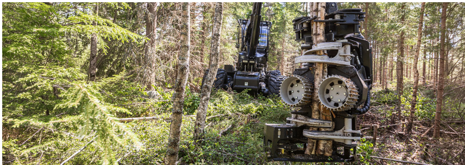
^ New TH52 with bunch processing device installed. Bunch processing is also available onto most of Logset TH harvester heads.
